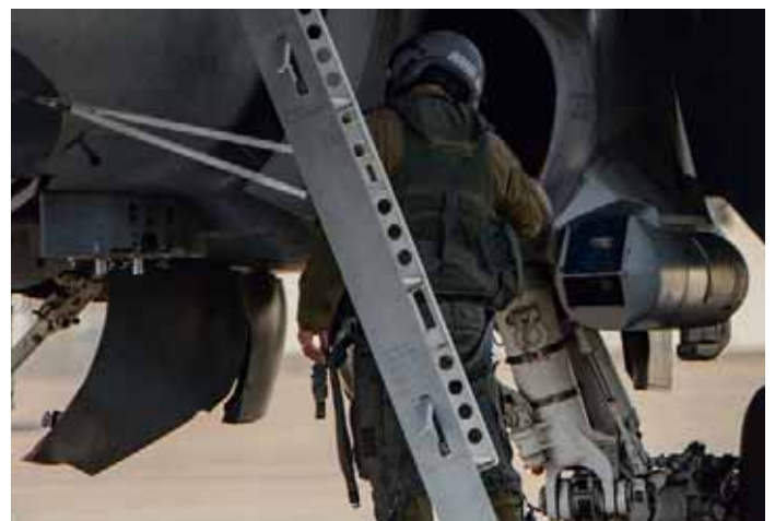
Sniper is currently carried on the side of the Hornet's intake, but will be moved to the centreline hardpoint
